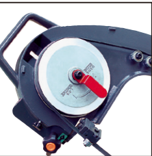
Fig. 2 Easy replacement of spare saw blade
